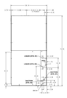
FIGURE 21 - LB360 PIPING CONNECTIONS
